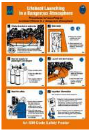
Lifeboat launching in a dangerous atmosphere
